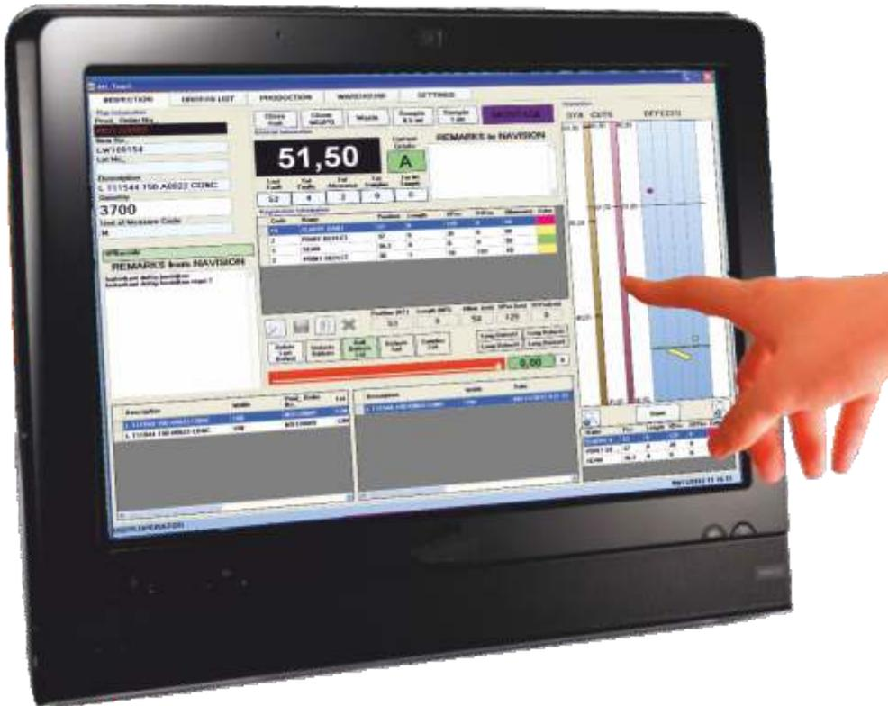
**ATF 750** is an integrated data logger for the textile industry. Input data, defect recording, printing function simply using the touch screen.
