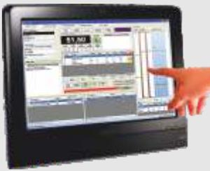
The operators inspect the fabric from big batch to big batch using a data logger ATF 750. The aim of the inspection process will be to obtain a map of the faults and of all the relevant features of each fabric batch. All the data of each inspected big batch are available for the next phase called «CUTTING OPTIMIZATION»
